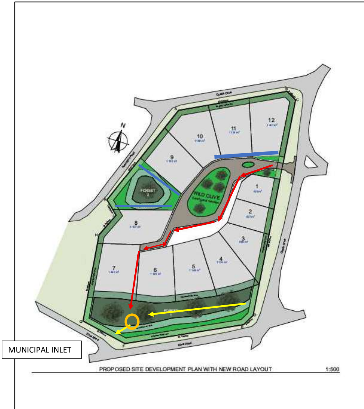
Figure 3: STORMWATER INFRASTRUCTURE PLACEMENT
